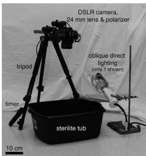
Figure 1. Filming arena and setup. Sterilite (Townsend, MA) tub dimensions (lwh) are 40 \times 33 \times 16 cm. DSLR, digital single-lens reflex.
